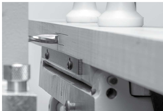
FIGURE 1. Align mortise by measurement or by adjusting to layout lines.
