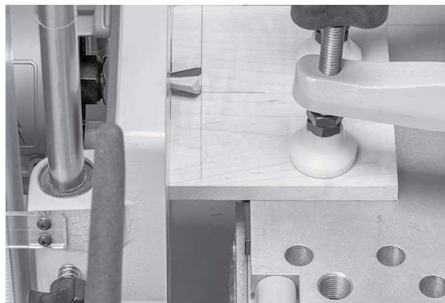
FIGURE 2. Set depth of cut to match the thickness of the joining material.
