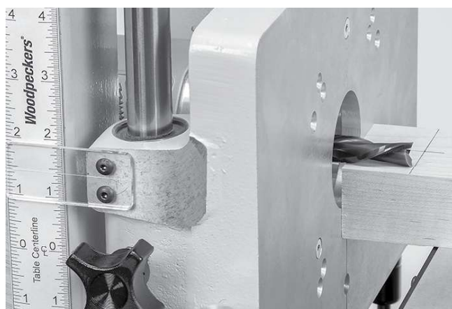
FIGURE 4. Adjust the depth of cut by adjusting the router.
