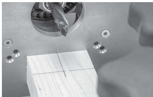
FIGURE 1. Carefully lay out the centerline of your stock and the depth of the tenon cut.
