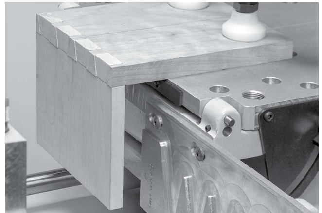
FIGURE 6. Make sure your dovetail test piece will fit over the rails so you can test in place. Sneak up on a perfect fit with small adjustments.
