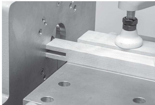
FIGURE 4. Bridle joint mortise cut with stock perpendicular to Vertical Table.
