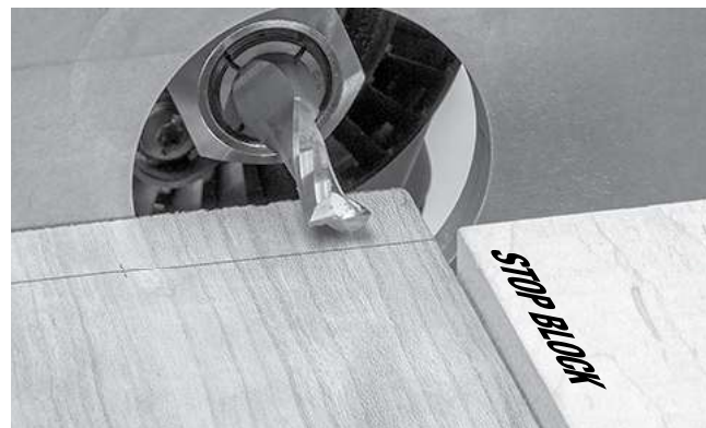
FIGURE 2. First cut in first board leaves a finger.
