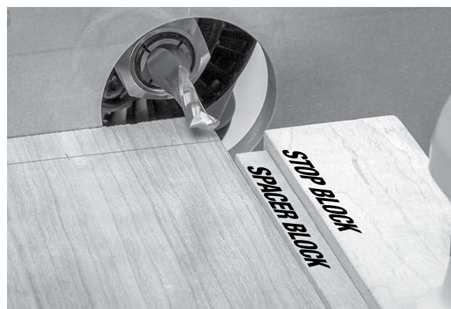
FIGURE 3. With spacer block in place, first cut on second board begins at edge to mate with first board.
